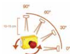
IP69K: High pressure, high temperature spraydown at multiple angles and rotation
