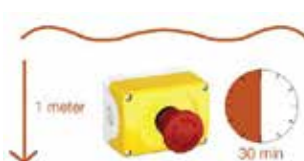
IP67: Submersion to one meter for 30 minutes
